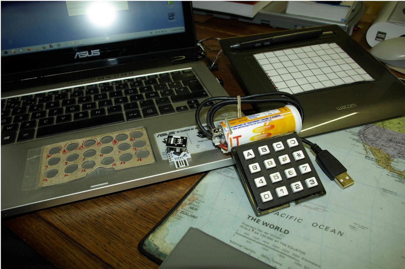
Here you see how I adapted my touchpad with a cardboard and tape on one side. The cardboard holes makes it easy , the thickness allows to touch and not generate a signal this gives a clear separation and distincting and feel where you can tap/touch.
